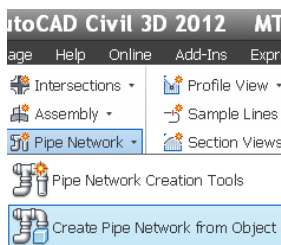
Figure 55 – Create a pipe object by creating a pipe network from a figure
