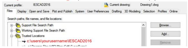
The MTO IESCAD 2016 system is now loaded and will stay loaded until you manually unload it or set your saved 'Profile' as the current profile.
